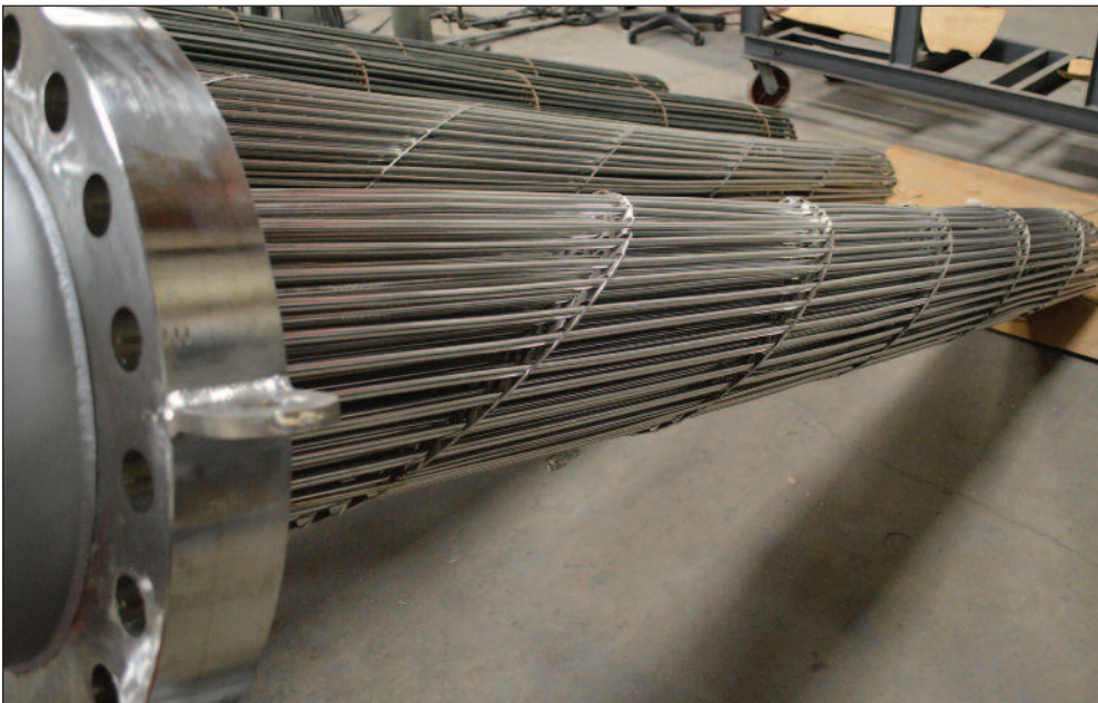
Angled turbulators - optimum heat transfer
