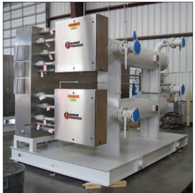
Diesel fuel oil heaters
