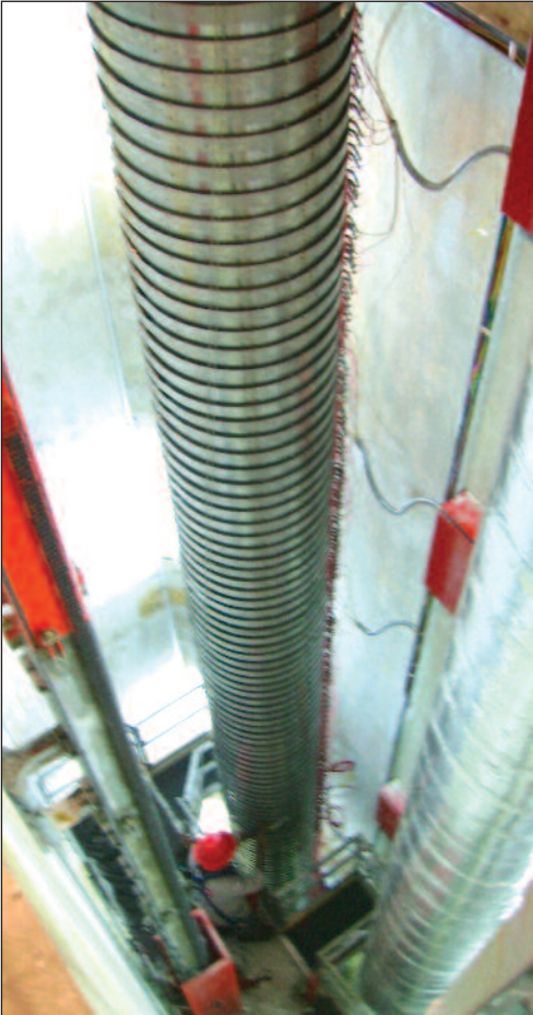
Band heaters - hydrotest chamber
