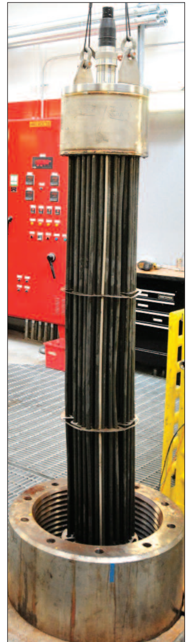
Subsea heater - 5000V, 3500m depth
